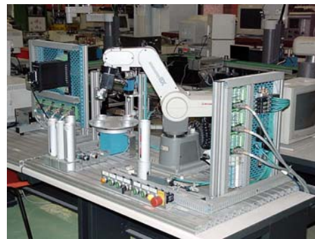
Fig. 11 Robot for assembling components
