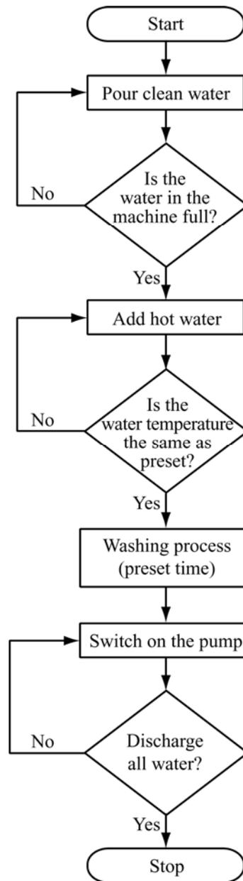
Fig. 20 Sequential control block diagram
