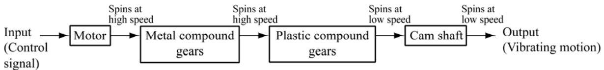
Fig. 22 Block diagram of a mechanical system
