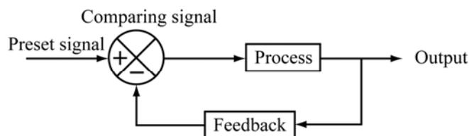
Fig. 14 Block diagram of a closed loop control system
