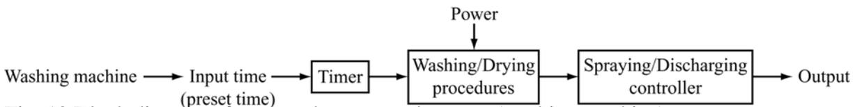
Fig. 12 Block diagram of an open loop control system (washing machine)
