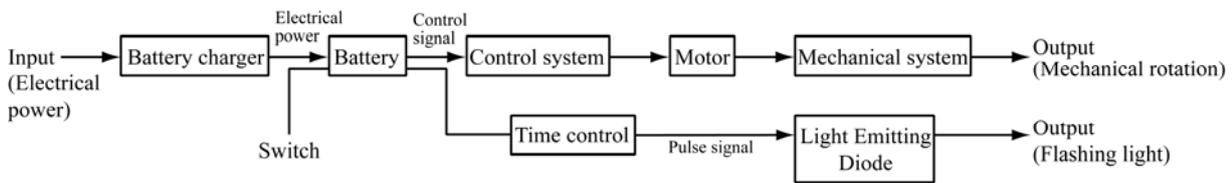
Fig. 21 Block diagram of an electronic control system
