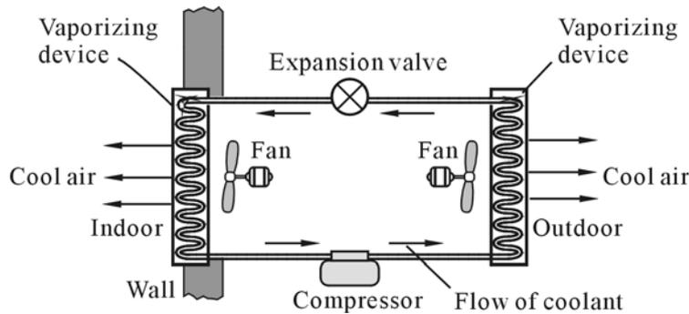
Fig. 17 Internal structure of an air conditioner
