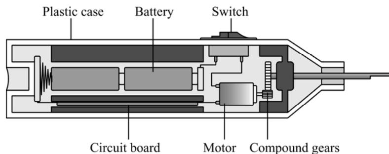
Fig. 23 Cross section of an electric toothbrush
