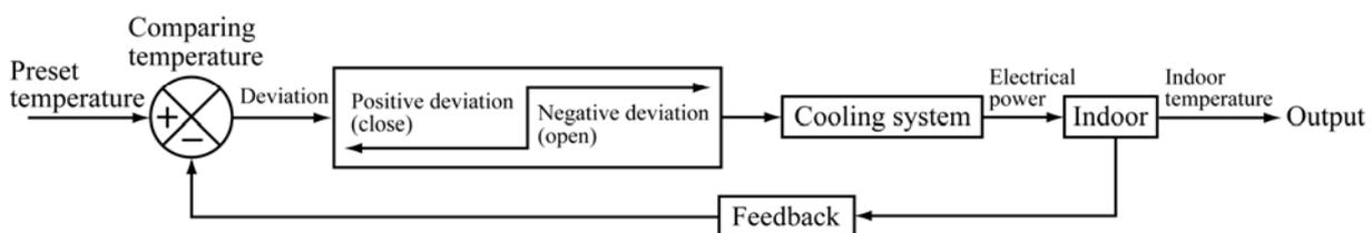
Fig. 15 Block diagram of the control system of an air conditioner
