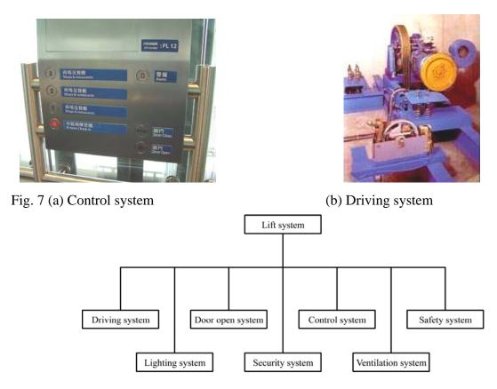
Fig. 8 Sub-systems in a lift
