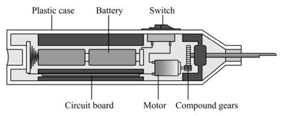
Fig. 23 Cross section of an electric toothbrush
