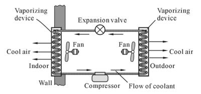
Fig. 17 Internal structure of an air conditioner
