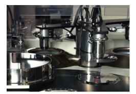
(a) Production line of CD-ROM Fig. 5 Examples of pneumatic systems
