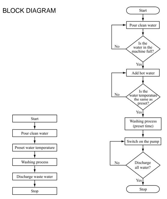
Fig. 19 Operation block diagram
