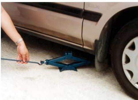
Fig. 1 (a) Car jack to multiply force
