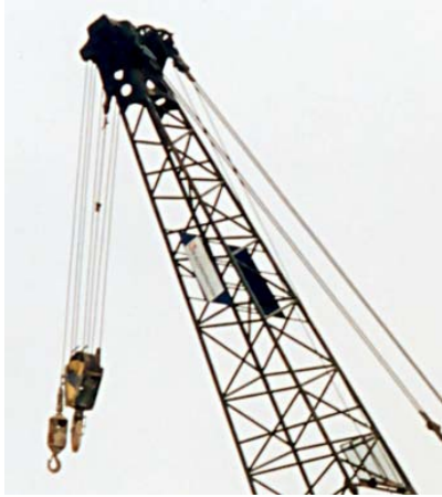
Fig. 10 Block and tackle system in the cranes
