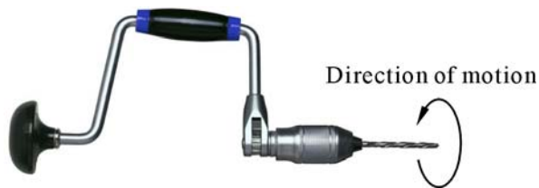
(b) The motion of the bit of a hand drill
